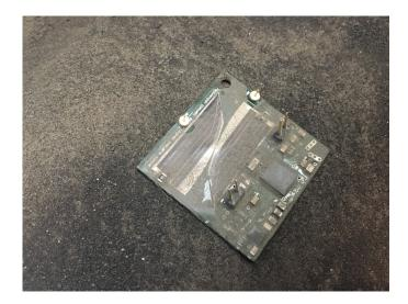
Figure 4.1: Impact test article on bed of lunar regolith simulant after exposure to 27,000 g's of acceleration to simulate impact with the lunar surface.
